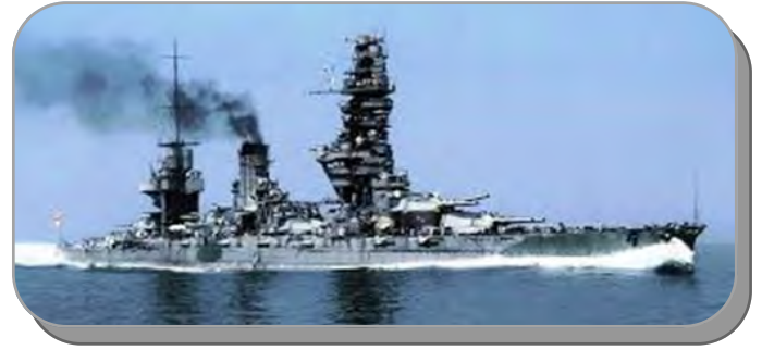
MASTRO DE PAGODE (PAGODA MAST)
